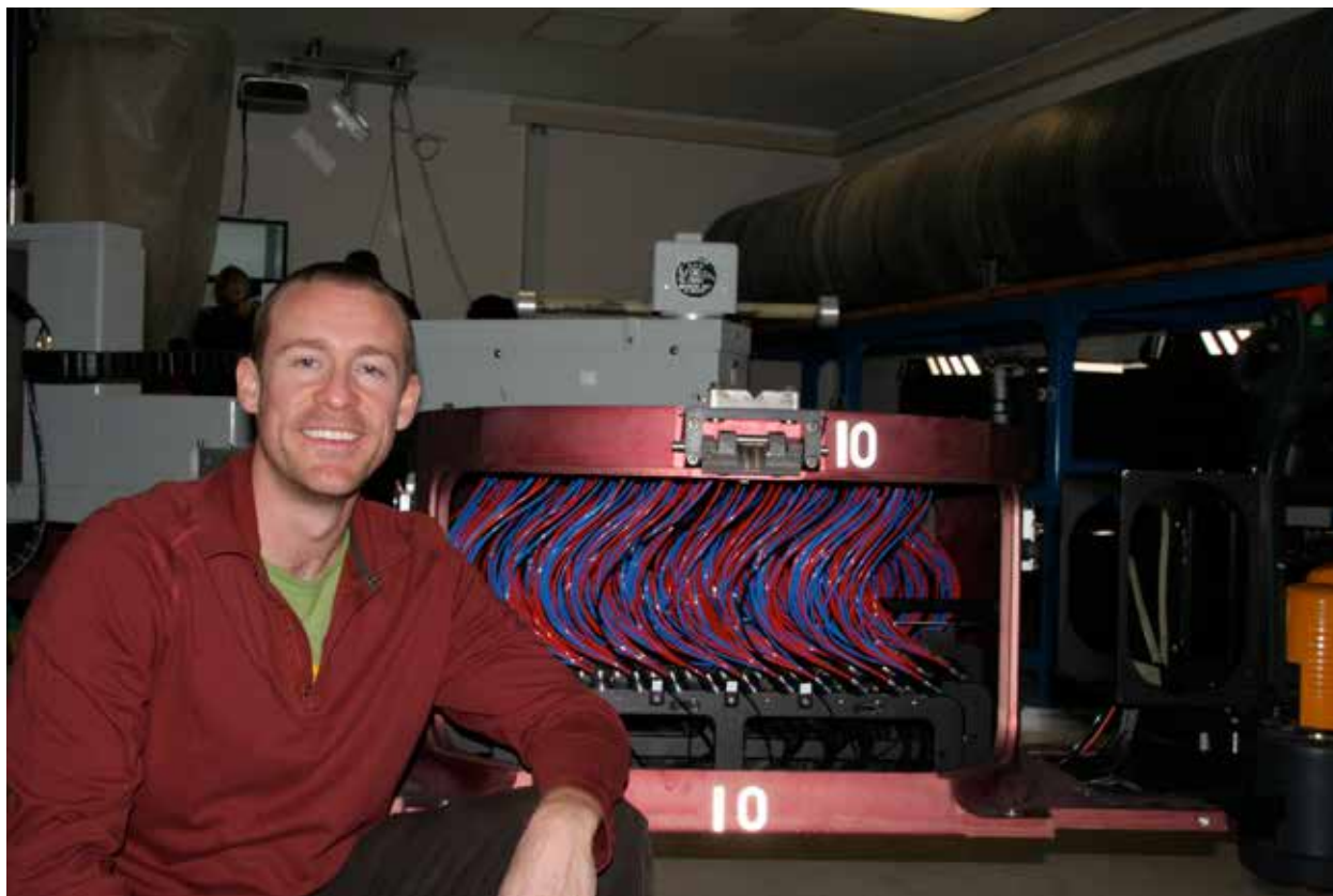
BOSS Survey Scientist Kyle Dawson poses in front of a 1,000-fiber spectrograph cartridge. The Baryon Oscillation Spectroscopic Survey (BOSS) is just one of four major astronomical surveys conducted as part of the third phase of the Sloan Digital Sky Survey. By mapping the spatial distribution of red galaxies and quasars, BOSS scientists aim to shed light on the formation and evolution of the universe. (PHOTO COURTESY OF SLOAN DIGITAL SKY SURVEY.)
