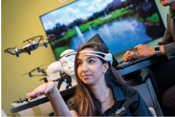
Sloan Scholar Sarah Garcia is pursuing her Ph.D. in computer science at the University of South Florida, where she is studying the brain computer interface, machine learning, and virtual reality. Here, Garcia wears an experimental device that reads electrical signals in her brain, allowing her to control the drone using only her mind. (PHOTO BY SANDRA ROA, REPUBLISHED COURTESY OF THE UNIVERSITY OF SOUTH FLORIDA)
