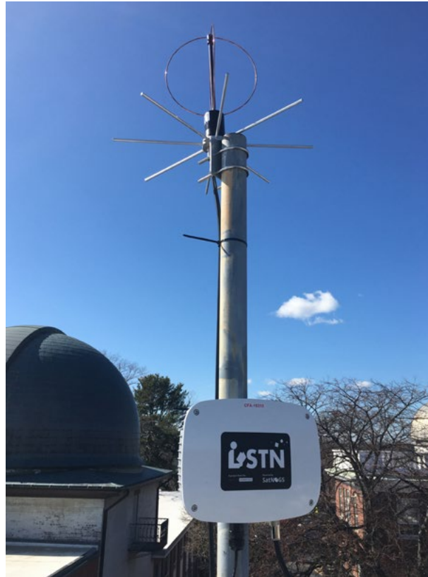
Installed on the roof of the John G. Wolbach Library in Cambridge, MA, this antenna is one node in a network of “ground stations” that receive research data from small micosatellites launched into orbit by scientists. A Sloan-funded effort by librarian Daina Bouquin is seeking to standardize and expand this network, with planned expansions at public libraries from Moldova to Texas. (PHOTO COURTESY OF JOHN G. WOLBACH LIBRARY, CENTER FOR ASTROPHYSICS | HARVARD & SMITHSONIAN. PHOTOGRAPHER: NICO CARVER)
