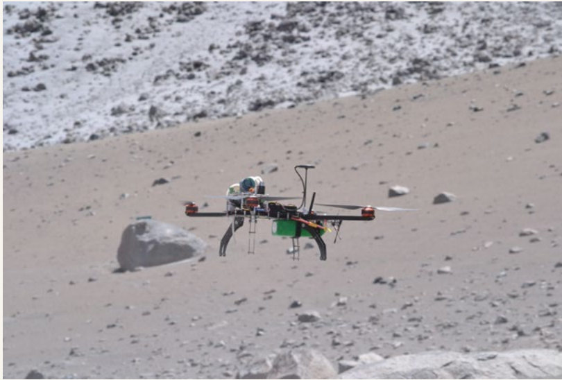
Technological innovation was an essential element of the DCO research agenda. Here, researchers perform a test flight of a MultiGAS-equipped Matrix Quadcopter. The drone, which measures atmospheric carbon, was used by DCO scholars during a 4,000-kilometer voyage from Peru to Chile that aimed to help quantify and model volcanic carbon emissions. (PHOTO COURTESY OF THE DEEP CARBON OBSERVATORY)
